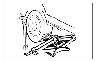
Lower the vehicle by attaching the folding wheel wrench to the jack and turning the wrench counterclockwise. Lower the jack completely.
